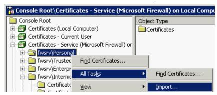
Locate the .pfx file and import it into this container. Once the import is completed, open
